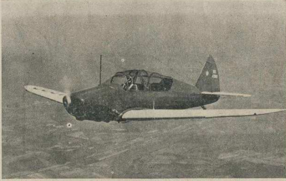
Still in experimental stage, Piper will eventually produce a four passenger low-wing with 125 mph cruise patterned after this thoroughly-tested Piper PT.
